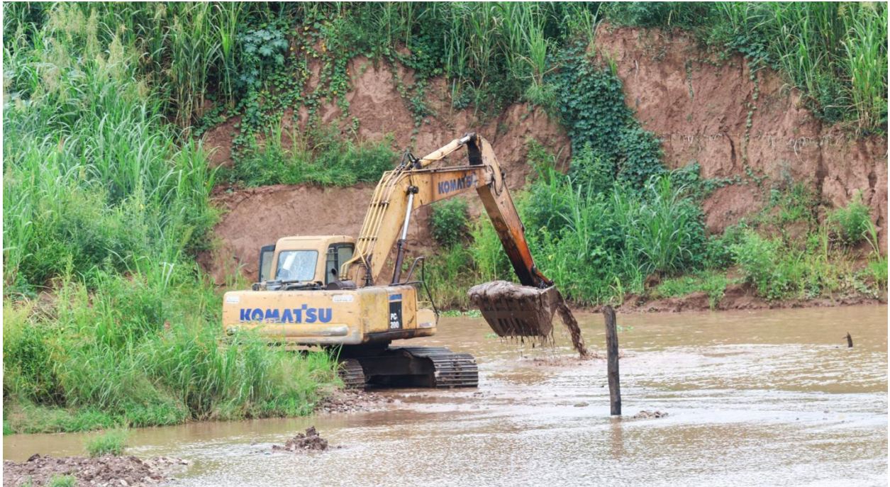
Along the Nam Tha River, small sand mining sites use excavator trucks to slowly dig the riverbeds for sand and also to remove bottom sediments and debris to keep the waterways deeper and navigable.
