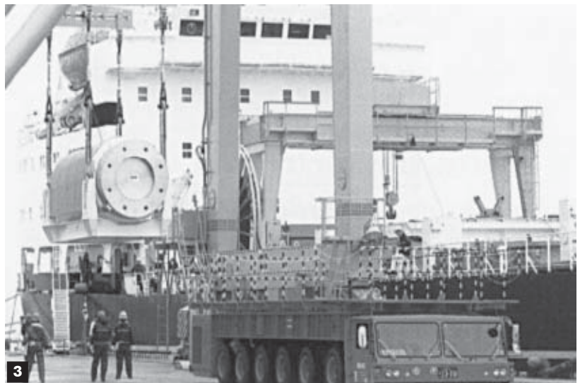
Unloading vessel for transport flasks.
