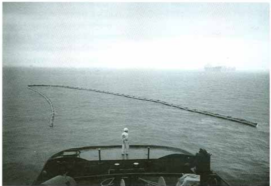
Deployment of boom as part of an oil spill response exercise (IMO/Singapore/TCTP OPRC Training, 25-29 October 1999).
