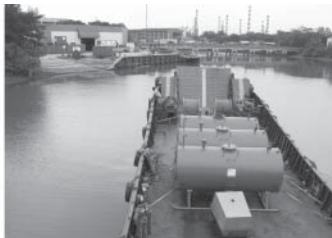
Skid tanks and booms loaded.
