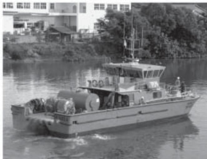
Skid tank installed on an EARL boat.
