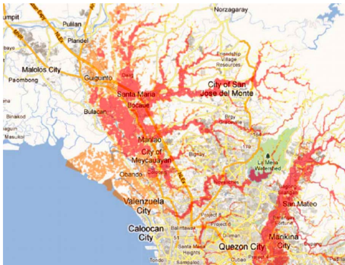
Figure 22. Flooding scenarios for large rainfall events.
