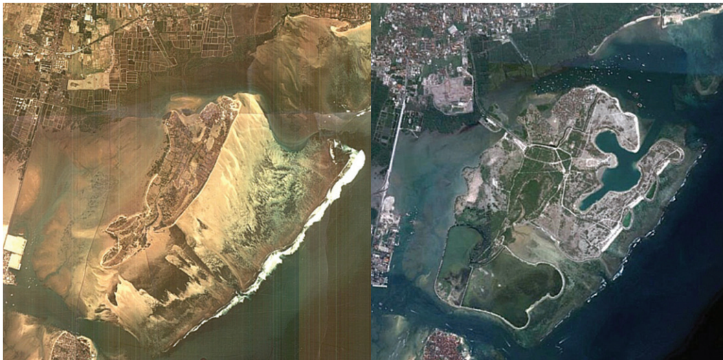
Figure 1. Serangan Island before (left) and after reclamation (right). The reclamation increased the size of the island by almost five times.
