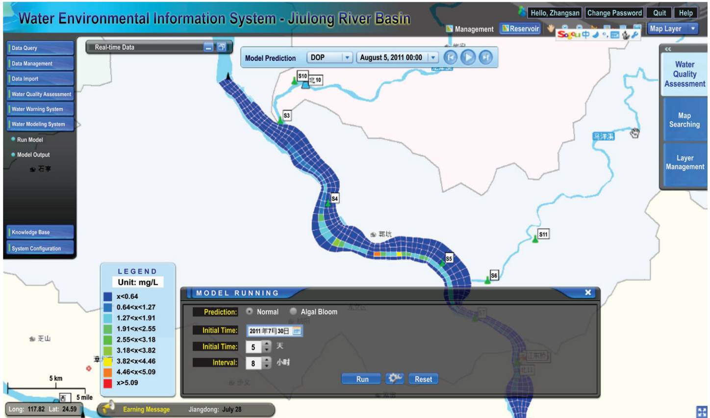
Figure 3. Model output shown on the JRWIS. A coupled model (SWAT+EFDC+WASP) was integrated into JRWIS to predict water quality. (This modeling work was completed by Dr. J. Huang of Xiamen University.)
