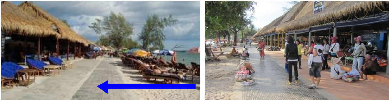
The buffer zone is the 10-15 m transition between easement and the built up zone. The walkway is part of the buffer zone. The trees lined up in this area were maintained to prevent erosion.
